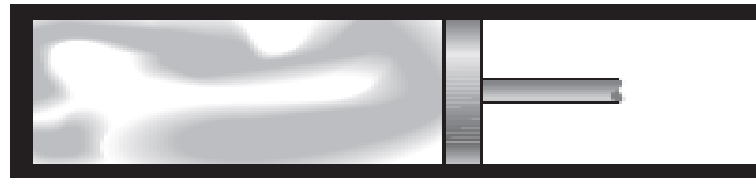
(b) Quasi-equilibrium expansion and compression of a gas
